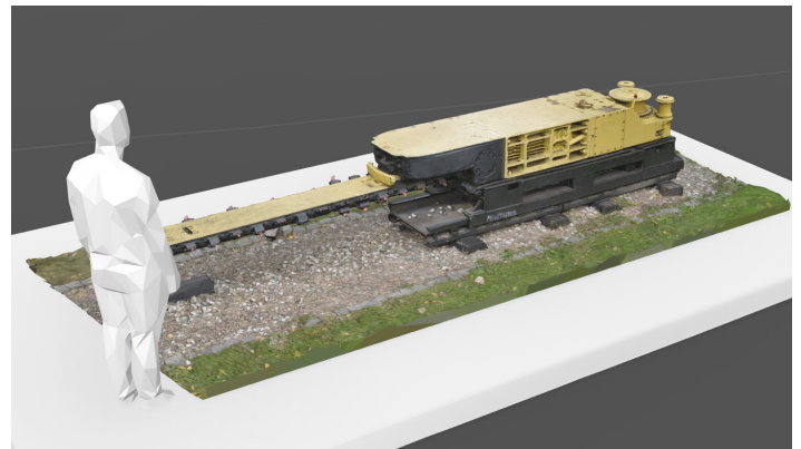
Figure 7. Screenshot from the 3D model of Frederick Hurda's first chain coal cutting machine located in Poland, which was used widely in English and German mines in the 19th century.
