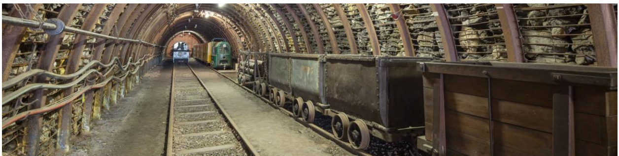
Figure 46: Underground gallery and narrow railway equipped with wagons and trolleys conveying coal to the surface (URL49)
