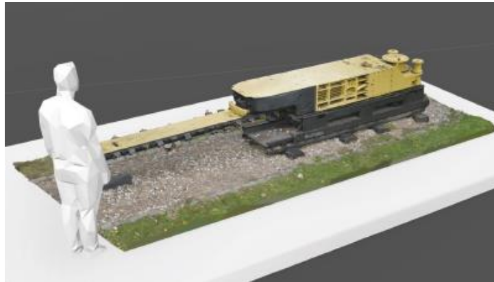
Figure 4.4 Screenshot from the 3D model of Frederick Hurda’s first chain coal cutting machine located in Poland, which was used widely in English and German mines in the 19 th century.
