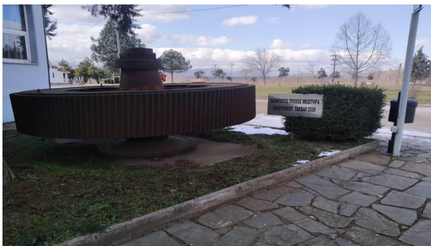
Figure 57. TAKRAF 2000 gear reducer toothed wheel, exhibit at the West Macedonia Lignite Centre (Giouvanidis, E, (2024) personal archive).
