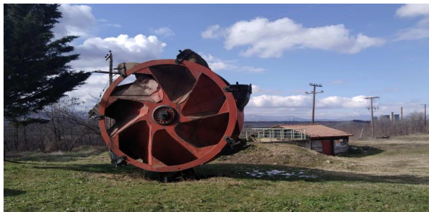
Figure 58. Bucket wheel, part of the excavators, exhibit at the West Macedonia Lignite Centre (Giouvanidis, E, (2024) personal archive).
